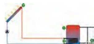
Internal heat exchanger, pump logic, return temperature maintenance (2 x E13170 additionally required)
