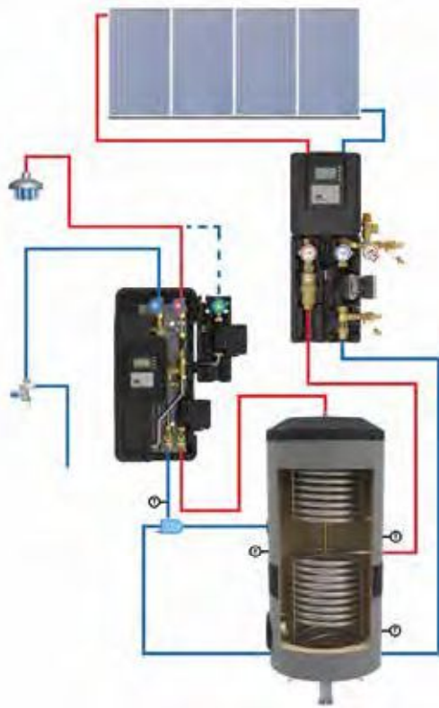
Mounting example SolarBloC midi Basic in combination with a FriwaMini with integrated circulation
