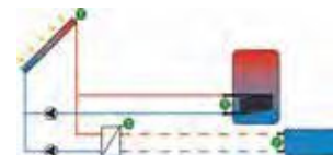
Storage tank and swimming pool, stand-alone operation of the external heat exchanger, pump logic (2 x E13170 additionally required)
